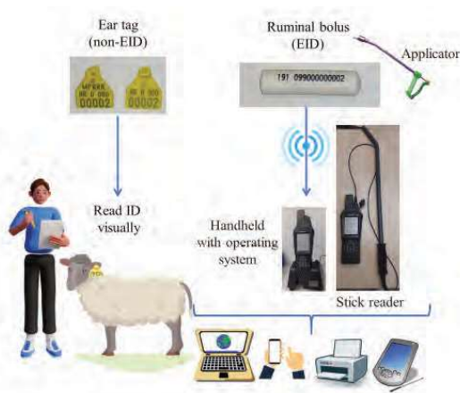
Figure 1. How application of electronic identification (EID) works in small ruminants
