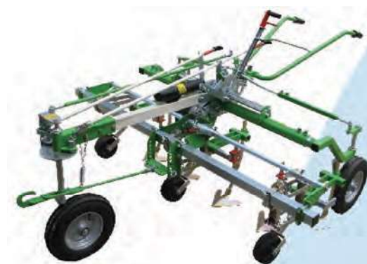
Figure 1. Newly developed inter-row cultivator
